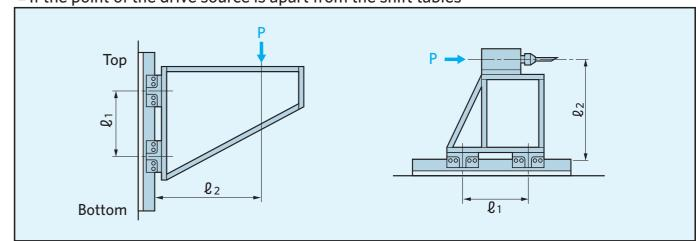
If the position of drive source P is apart from the rail surface by  $\ell_2$ , of  $\ell_2/\ell_1$  exceeds 1.67 when the coefficient of friction  $\mu$  is 0.3, resulting in malfunctioning. Take the allowable moment load into consideration and reduce  $\ell_2/\ell_1$  below 1.5.
