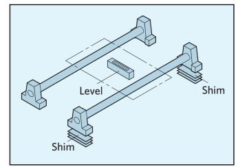
Select the B type if the parallelism t exceeds 0.3. Insert shims under the shaft holders to adjust them.
