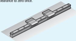
2) Fasten the mating plate to the shift tables finally, adjust the linear accuracy, and adjust the clearance.
