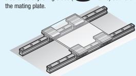
4 Adjust the clearance on the datum-side shift tables.
