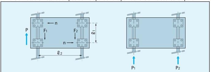
If the \$\mathcal{L}\_2/\mathcal{L}\_1\$ ratio of dual-axis parallel rails is large, the couple of the drive source P and resistance F1 and F2 becomes large and the slide shifter works improperly. Reduce £2/£1 below 3. As the point of the drive source becomes apart from the center, the condition becomes worse. Synchronize the drive source with P1 and P2 if  $\ell 2/\ell 1$  is inevitably larger than 3 for reasons of the structure.
